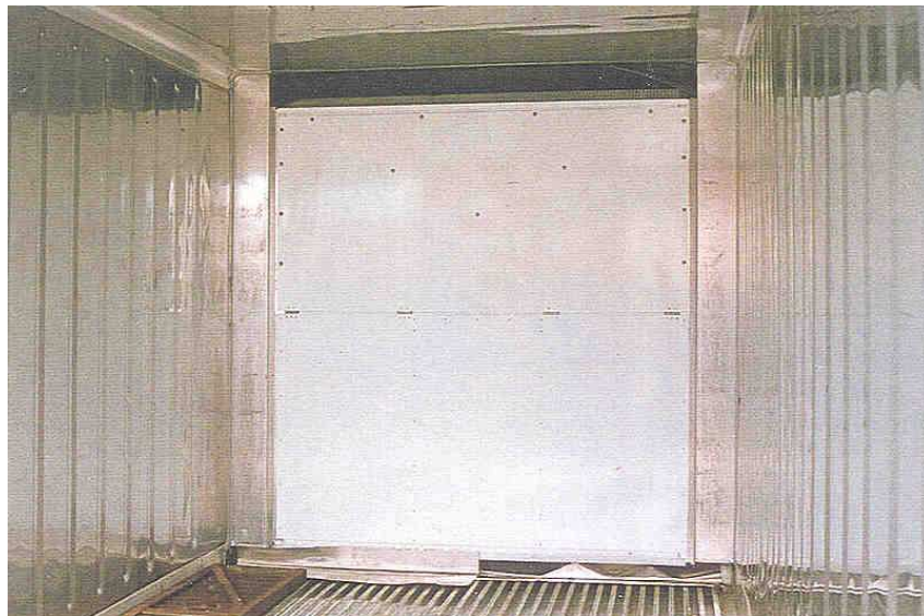
Top panel can be unscrewed giving access to refrigeration unit.
